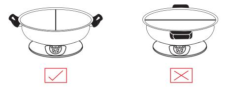
2. The pot will stick on the heating board tightly when heating. Do not remove the pot from heating board before cooling. Remove with force will damage pot and heating board.
